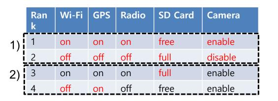
1) Normal scenario Active Wi-Fi, GPS, Radio=on, SD card = free, Camera = enable Exceptional scenario Inactive Wi-Fi, GPS, Radio=off, SD card = full, Camera = disable
